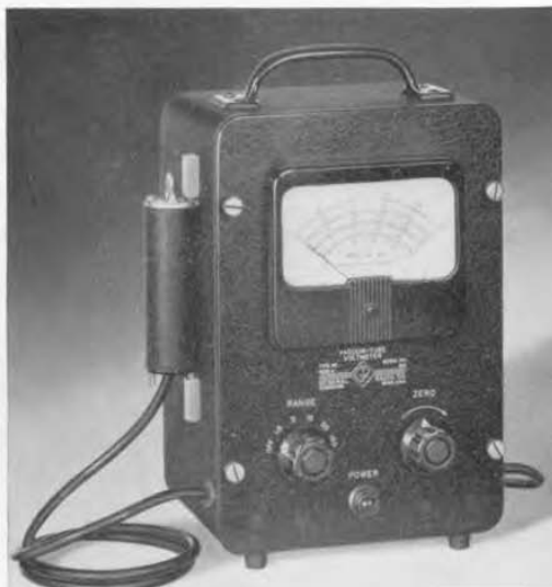
Figure 1. Panel view of the Type 1803-A Vacuum-Tube Voltmeter, showing how probe can be stored on side of cabinet.
